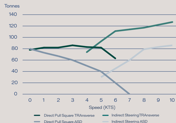
Direct and indirect Steering comparison between TRAnsverse 32m and ASD 32m
