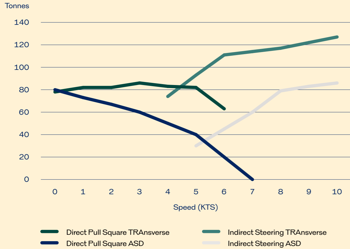
Figure 8A Direct and indirect Steering comparison between TRAnverse 32m and ASD 32m
