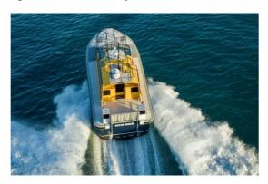
• Launches / work boats. There are a range of multi-role work boats that are commonly in use around a port. Line boats are sometimes engaged to transfer the inbound ship's mooring lines to the dolphins (mooring securing points). Work boats can also provide a platform to perform maintenance to port infrastructure and as a platform for diving activities. These types of work boats can vary from 9 meter to 20 meter in length and are propelled by conventional propellers and rudders.
