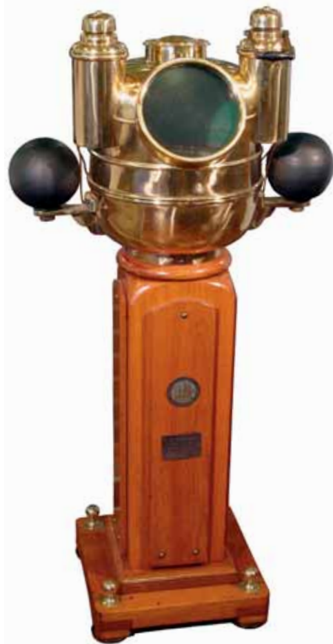
Compass binnacle made by Iver Weilbach & Co, instrument makers of Copenhagen. A non magnetic stand houses the compass and is mounted on gimbals. The balls on each side are correction balls which are moved in or out to correct the compass direction by counteracting the ship's magnetic field. The two canisters at the top contain lights to allow the compass to be used at night.
